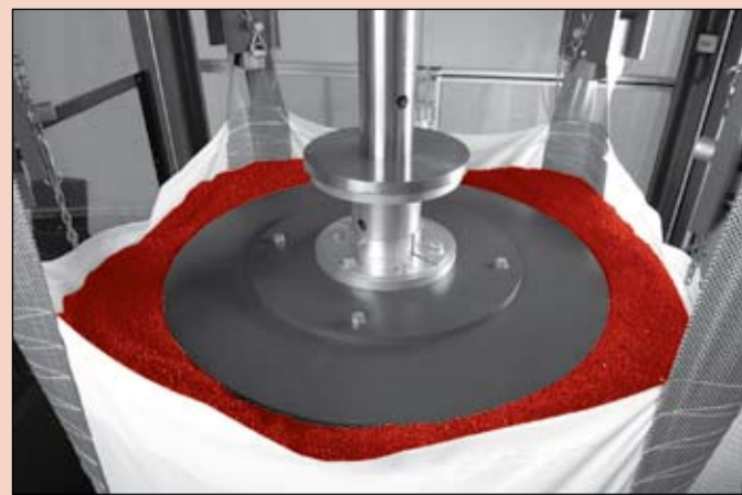
Top lift test of a four-point FIBC on the stacoTEST FIBC test rig in the Starlinger testing facility in Weissenbach, Austria.
