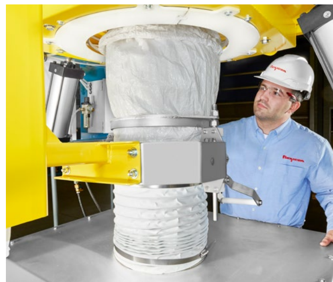
Complete discharge of material from bulk bags is achieved through the dual action of steel plates that press against the bottom seam while raising the bag (left), combined with a telescoping tube and clamp lock that pull the bag spout downward (right)
