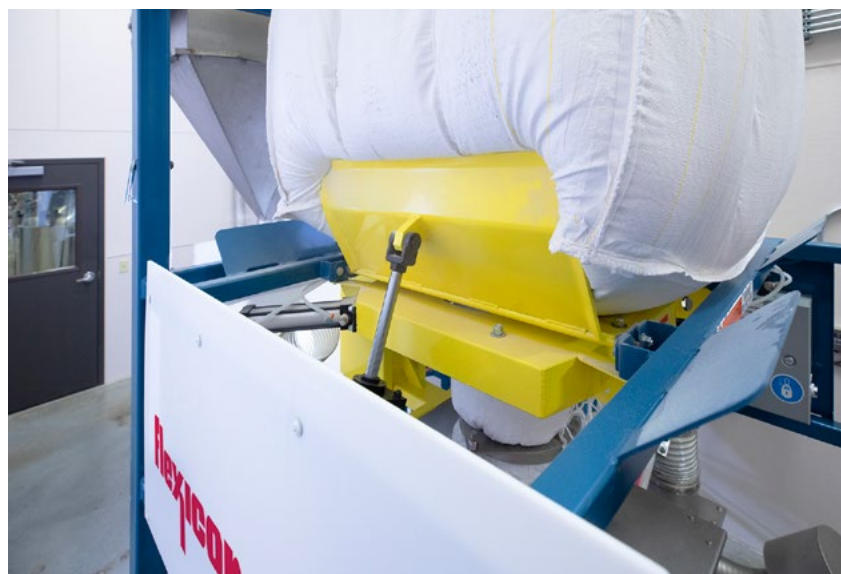
Complete discharge of material from bulk bags is achieved through the dual action of steel plates that press against the bottom seam while raising the bag (left), combined with a telescoping tube and clamp lock that pull the bag spout downward (right)
