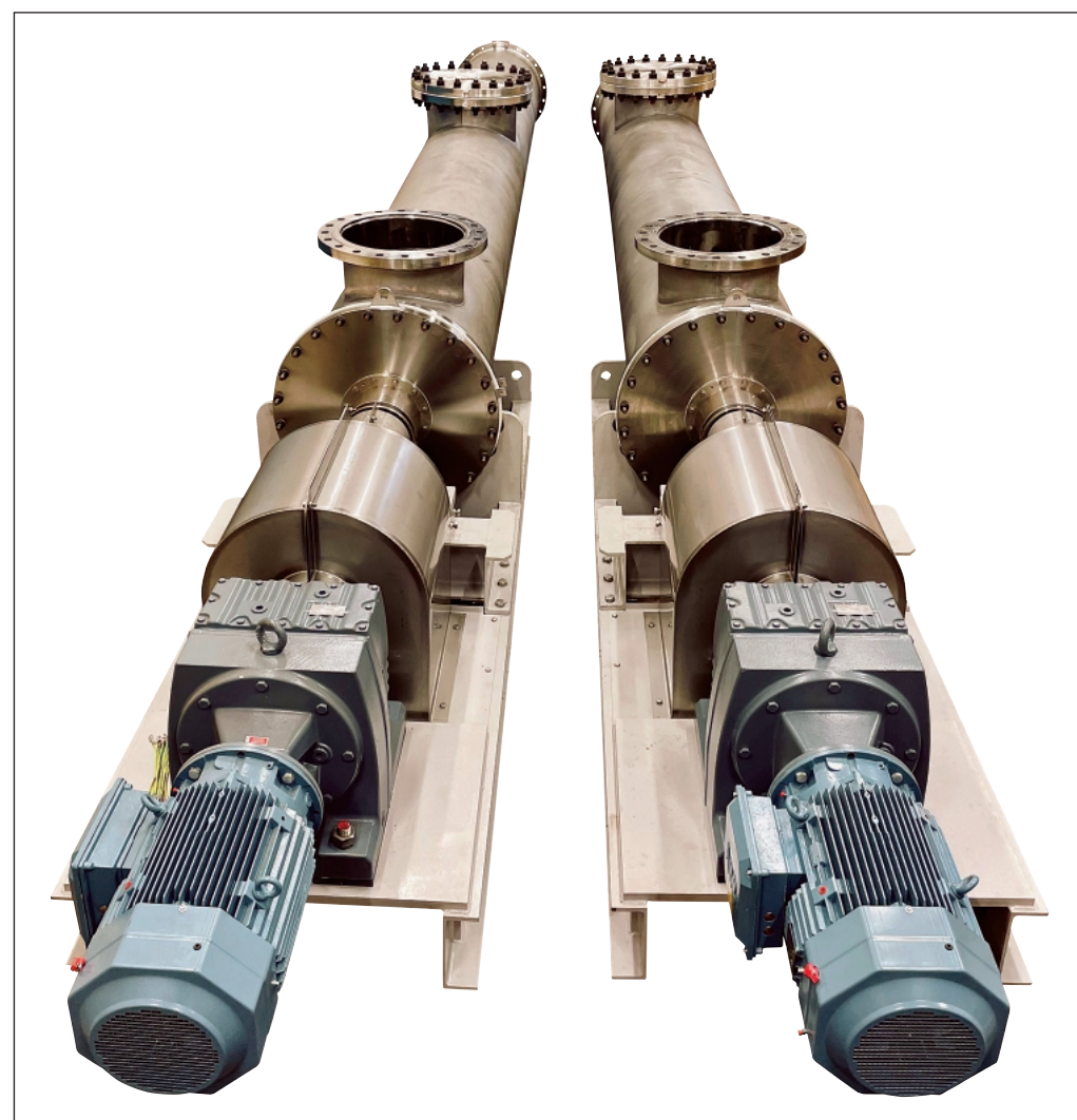
Carefully selected flights prevent cohesive powder from building up in Indorama's screw conveyors.
