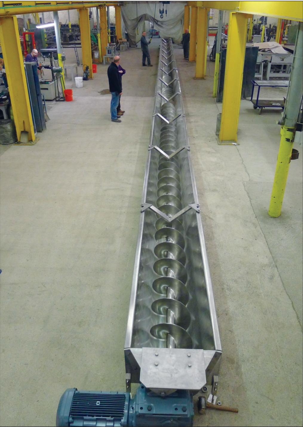
Long screw conveyors present a number of design & manufacturing challenges.
