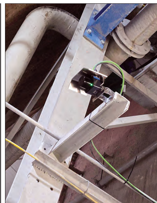
The Owl Eye LiDAR sensor: material flow monitoring for bulk handling operations (see p9).
