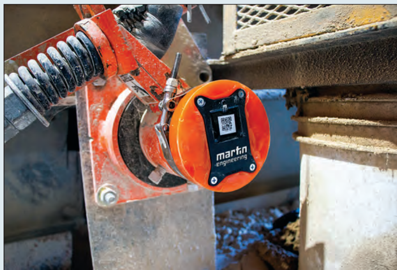
The CleanScape primary cleaner takes up less room and requires less maintenance than standard cleaners.
