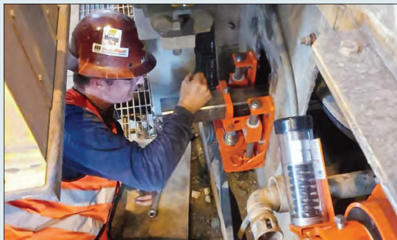
Safe maintenance on a belt cleaner system requires training and adherence to the proper safety procedures.
