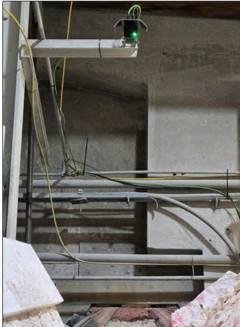
The Owl Eye LiDAR sensor above a conveyor belt.
