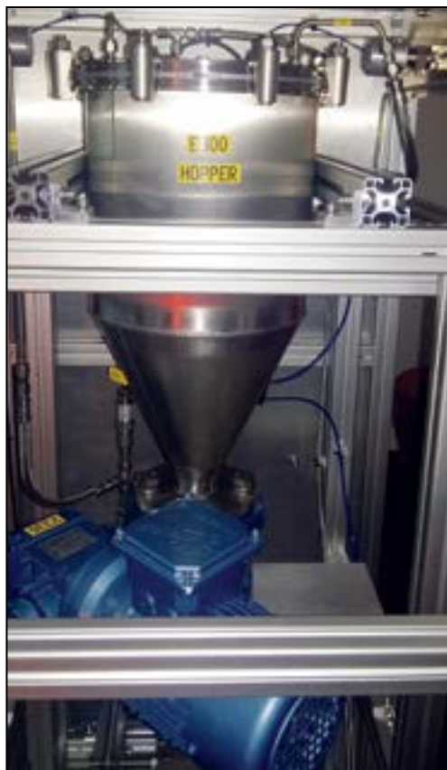
Ajax's equipment hopper provides a practical storage solution for prototype Sublimation System (see p13).
