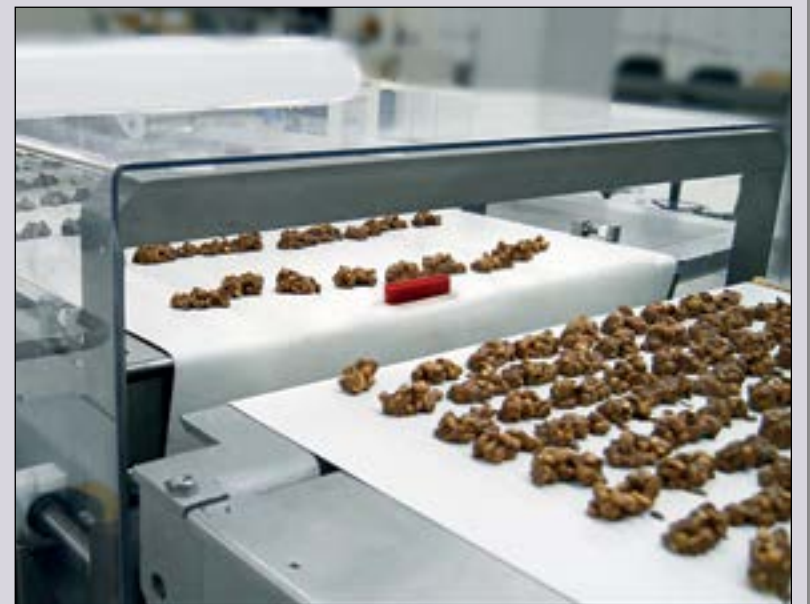
Conveyor-based systems require checks across the entire product path to confirm detection and rejection reliability.
