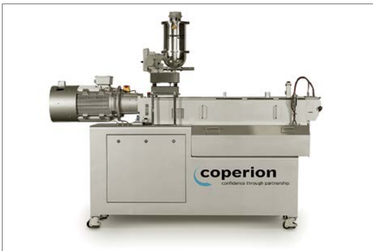
The twin screw extruder plays a central role in the research.
