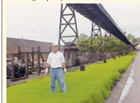
Grass started growing again under the primary raw material supply belt after the dust and spillage were eliminated.
