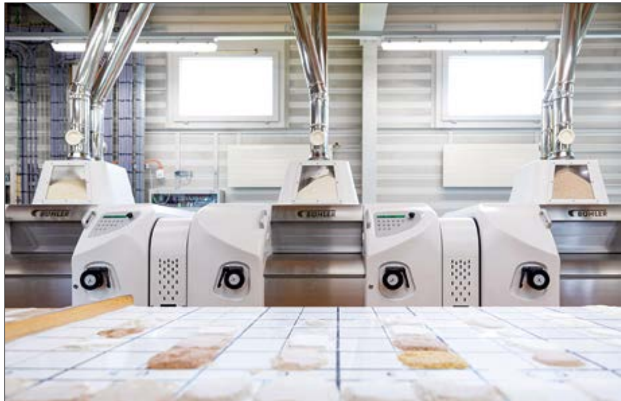
With a daily capacity of 24 tonnes, the fully automated training mill offers the opportunity to conduct training at an industrial scale.
