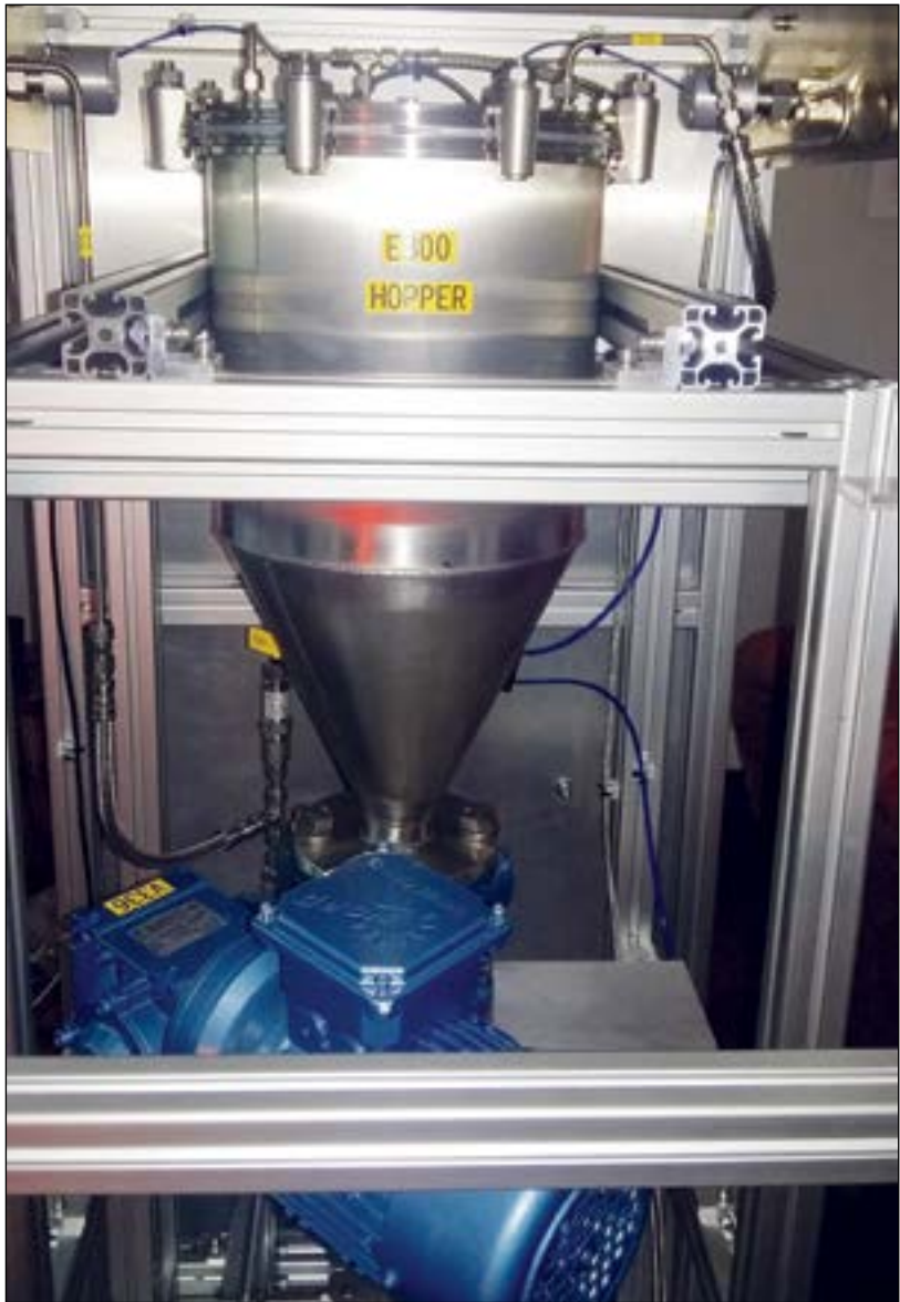
The stainless steel conical hopper has gas purge capability.
