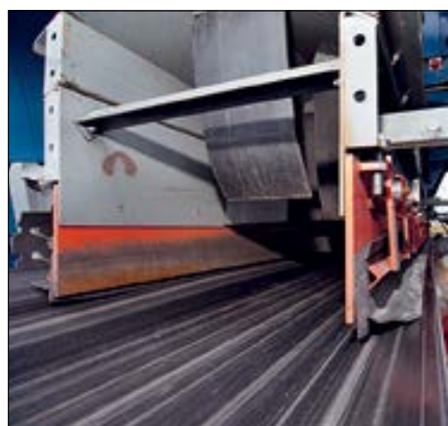
A properly structured enclosure is slightly elevated, with dust curtains, an external wearliner, and adequate skirting.
