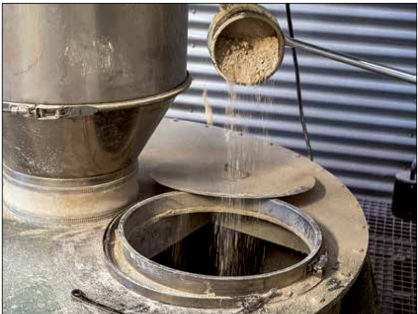
The new circulation system at the TestCenter allows different products to be combined with one another and accuracy tests to be carried out using different measuring principles.
