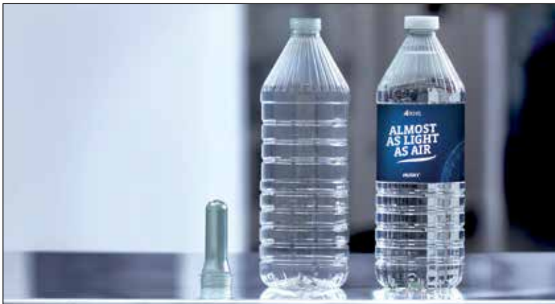
Consistent concept: from preform through blown PET container to filled, labelled and capped bottle.
