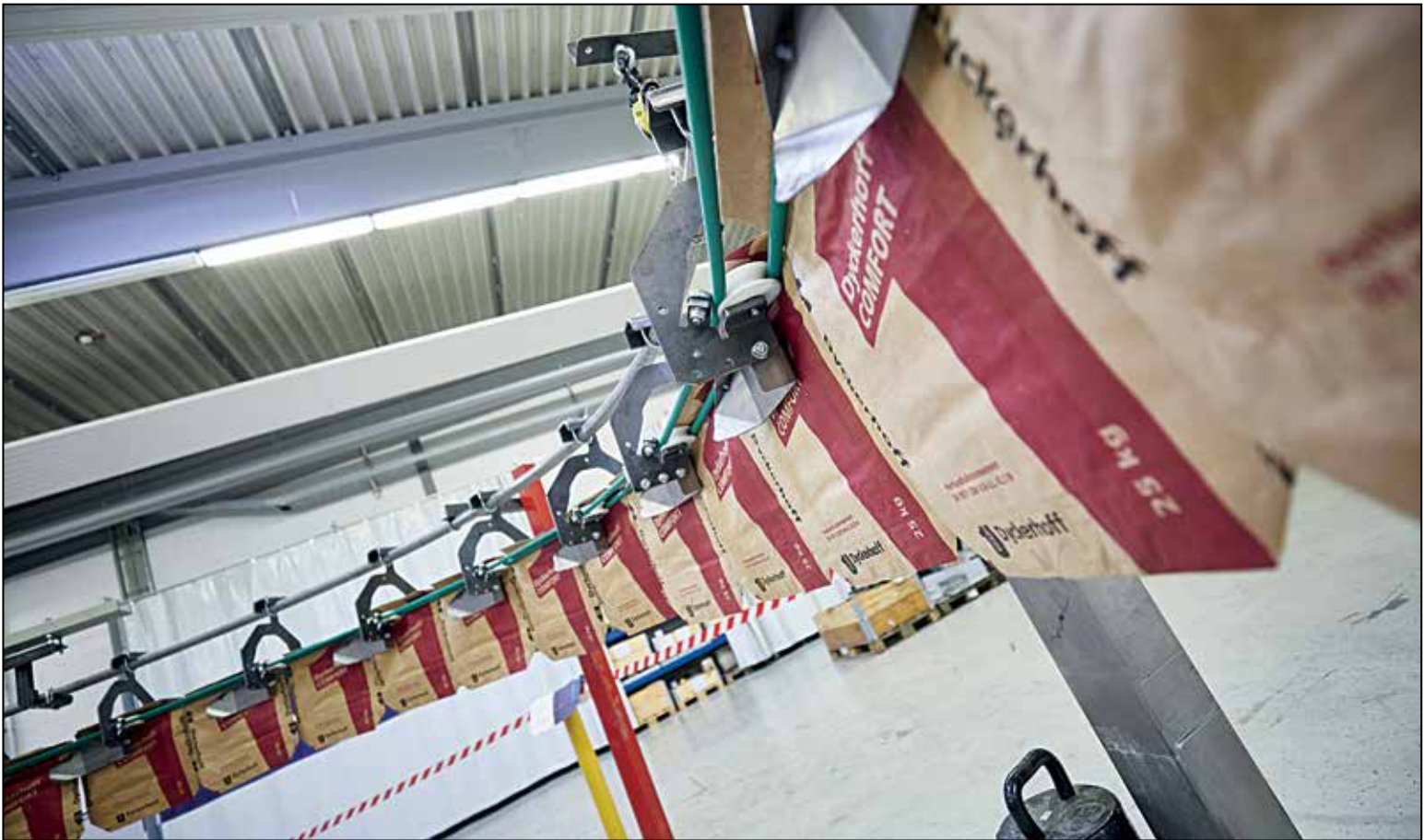
Haver & Boecker's new Radimat Pathfinder transfers bags from the Radimat – a bag separation and feeding device – to the Roto-Packjer automatic packing machine (see p3).
