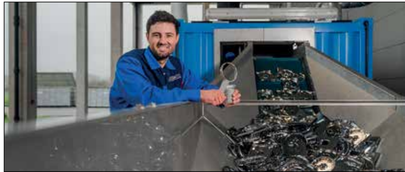
As the galvanised parts to be recycled are of different sizes and complexity levels, the first container deals with pre-shredding and includes a screening column.
