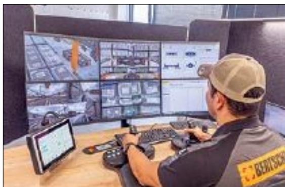
Bertschi employee remote operating the gantry crane of the Antwerp Zomerweg Terminal from nearby office.
