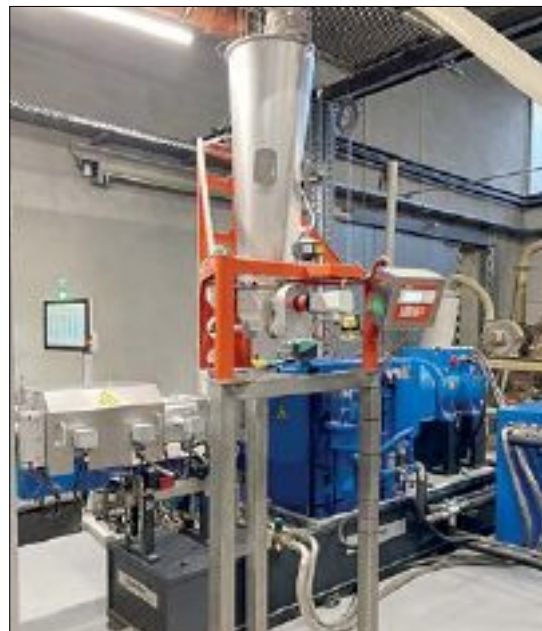
The Düngemittelwerk Coswig company has expanded production of fertiliser spikes with a Coperion ZSK extruder, equipped with a ProRate PLUS-MT twin screw feeder.
