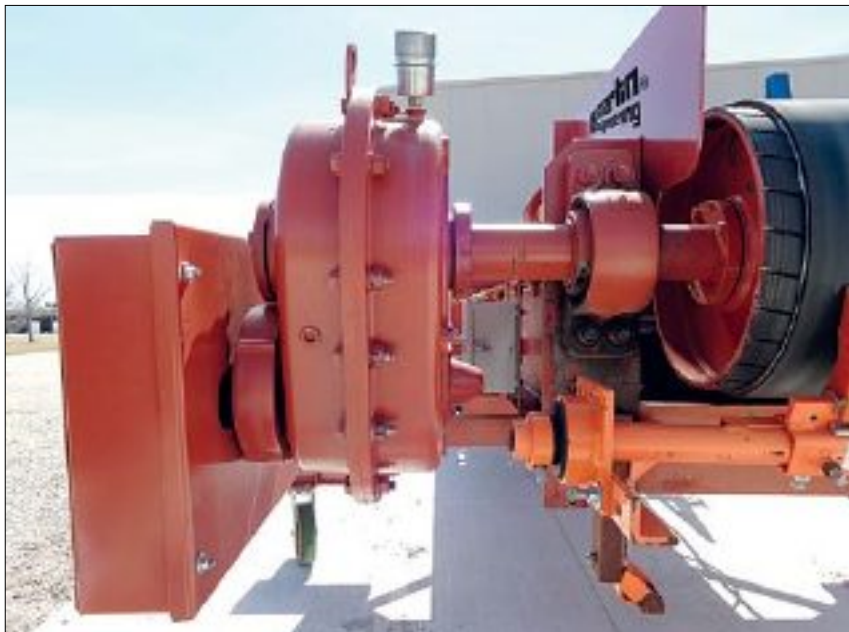
Conveyor drive motors can be as large as 600 HP (450 kW), moving belts as fast as 2000 fpm (10 mps).
