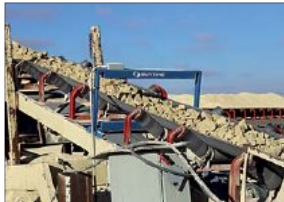
TN77 Metal Detector operating in an aggregate quarry.
