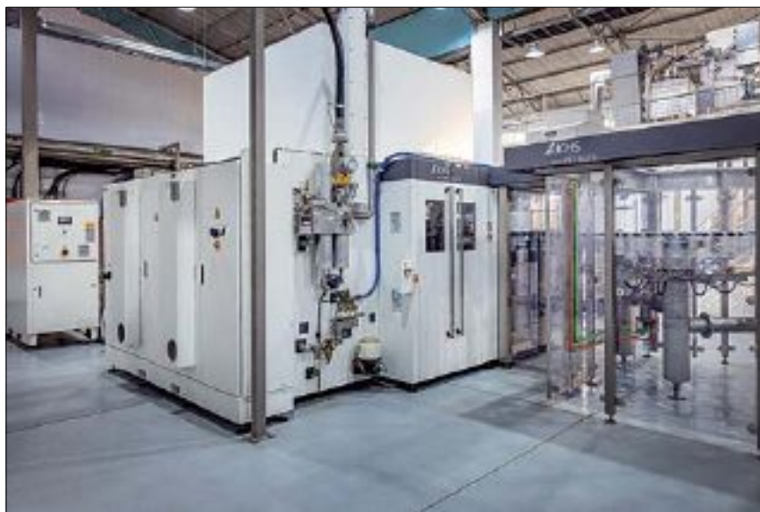
Stretch blow molder and filler in one: the InnoPET BloFill block from KHS allows up to 36,000 containers to be manufactured and filled per hour.
