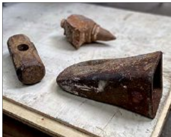
Typical tramp metal separated by a magnetic separator.
