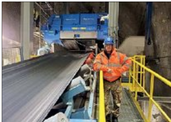
Electro Overband Magnet installed in a gold mine.
