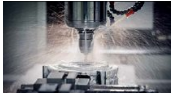
FA milling tool removes metal chips from a workpiece.
