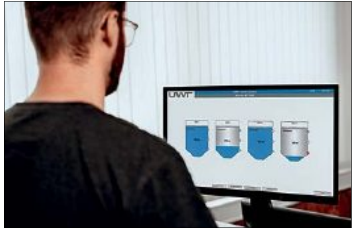
The NivoTec NT 3500 is a level visualisation system for displaying and monitoring fill levels and limit levels.
