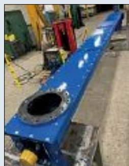
The screw conveyor is part of a new plant at Hubron.
