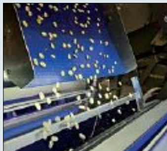
The system identifies and removes undesirable product defects and foreign material.
