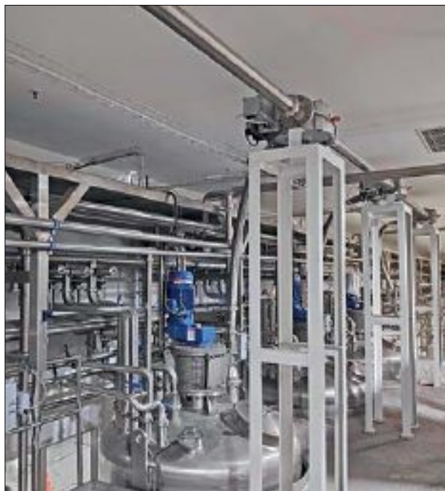
Liquid mixers with pneumatic feeding of salt.
