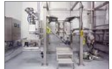
The finished mixture is filled into Big Bags by means of two HECHT filling stations.
