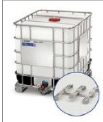
The 3-skid steel pallet with embossed sheet metal skids has an additional central skid compared to standard steel skid pallets. This ensures improved weight distribution thanks to a wider contact surface.
