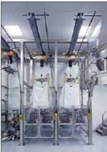
The Big Bags can be connected without danger of product contamination.
