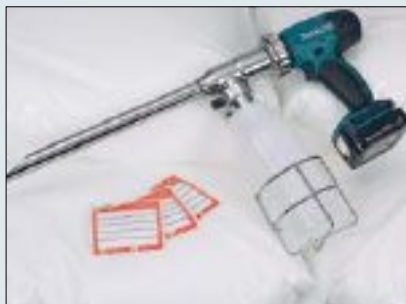
The lance tip is specially designed for good gliding and easy penetration into the material.
