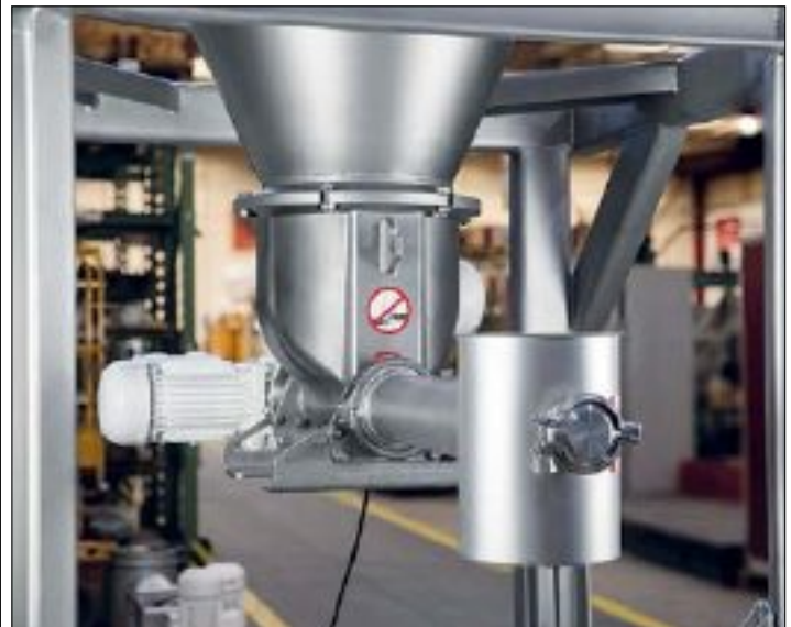
Gercke's FEEDOS M is a high-precision feeding and dosing device for medium capacities between 20 and 3600 l/h. (see p7).
