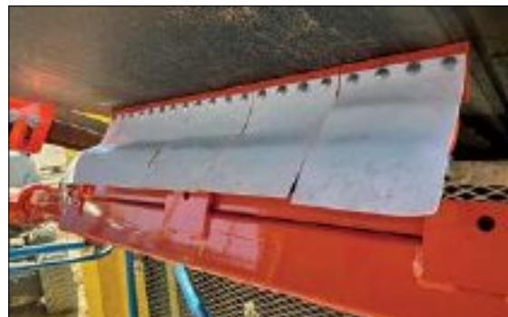
Slick heavy duty deflector shields improve performance from wet applications that experience buildup.
