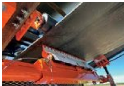
The mounting assembly firmly secures the secondary cleaner to the stringer.
