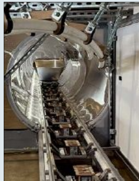
Magway's technology enables control over the horizontal and vertical movement of loads up to 250kg, with a throughput capacity of 1,000 tonnes per hour.
