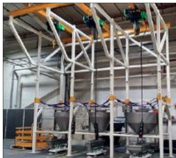
The first step in efficient bulk material handling is the use of specialised equipment such as big bag dischargers.
