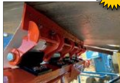
Cartridges with individual tensioning improves cleaning efficiency and effectiveness.
