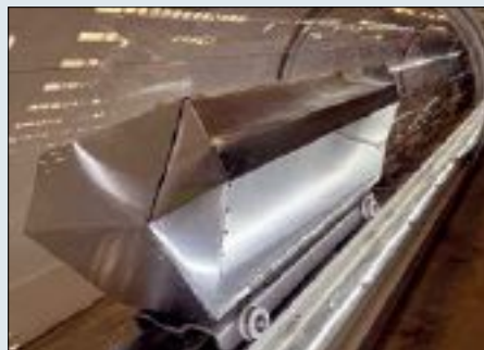
Magway's magnetic propulsion bulk material handling technology.
