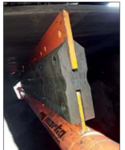
Martin's SQC2 Secondary Belt Cleaner features a unique slide-in/out assembly for safe and easy blade replacement.
