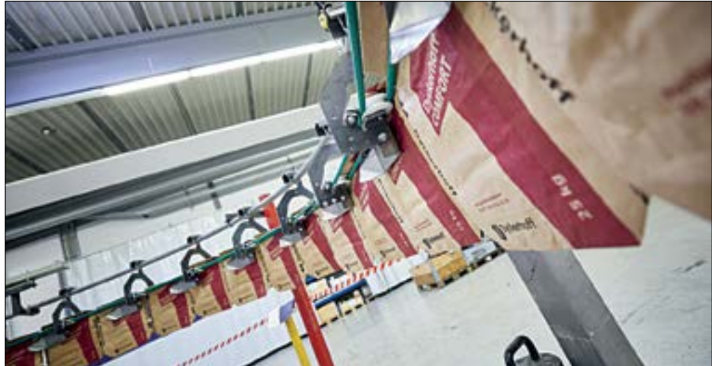
Haver and Boecker's Pathfinder transfers bags from the Radimat — a bag separation and feeding device — to the Roto-Packjer automatic packing machine (see p13).
