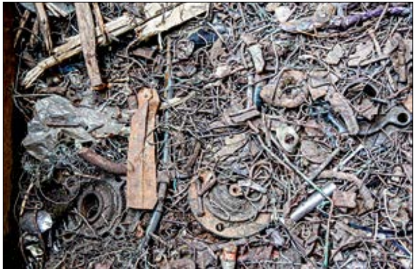
Separated tramp ferrous metal.
