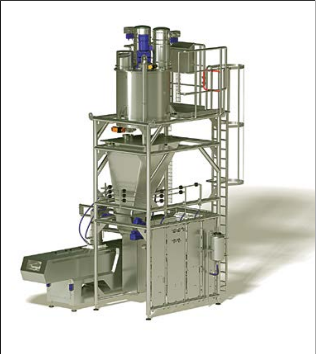
Zeppelin's Codos system continuously doses, mixes and kneads solid and liquid Components (see p7).
